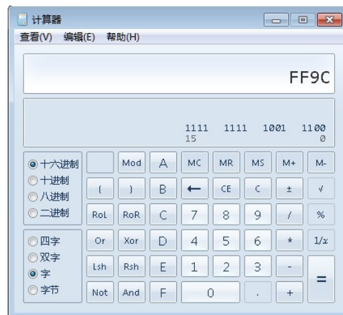
picture9.8 "-100" Convert to short type and display in hexadecimal
