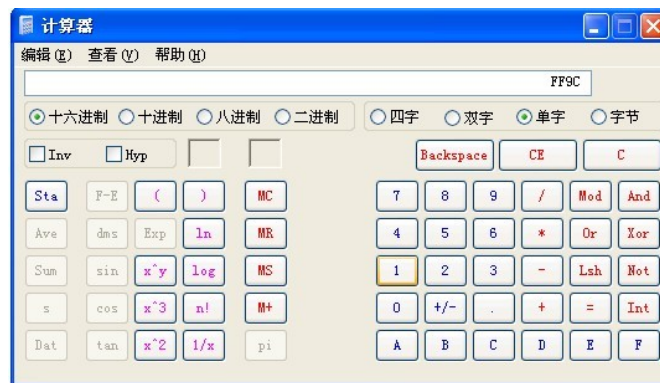
picture9.4 "-100" Convert to short type and display in hexadecimal
